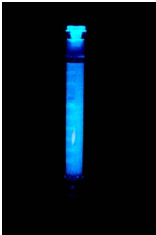
Figures 3 and 4. Fluorescence emission image of dialyzer probe under laser excitation (355 nm) (left) and spectral emissions derived from the spectral imagery.
